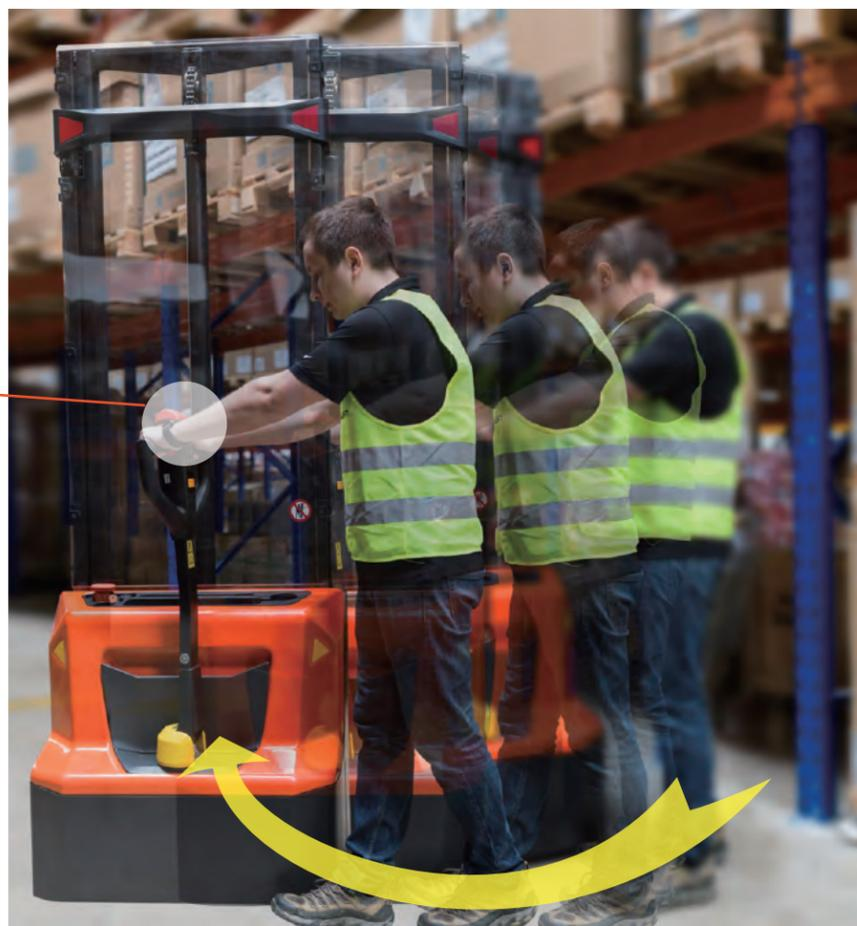
The tiller bar is supported by the air spring which helps to return the tiller to its vertical position without strike in the end point.
