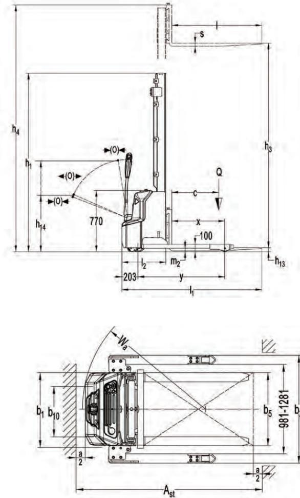
Type sheet for industrial truck acc. to VDI 2198)
