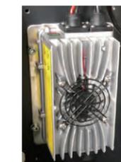
For PSE12B the charger with current 12A is used. The standard charging time is 7 hours
