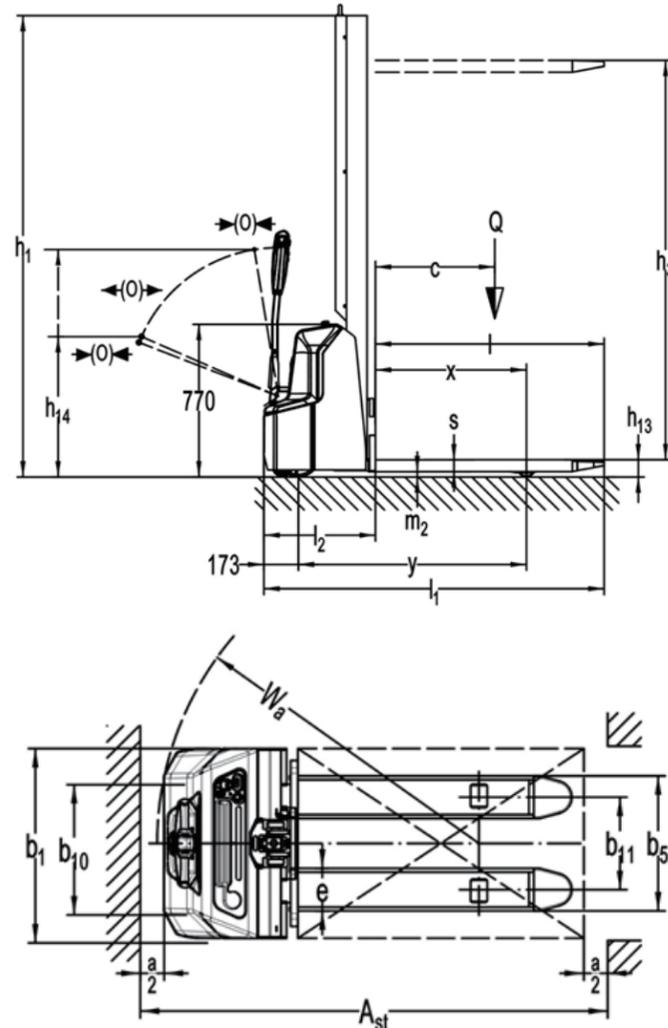
Type sheet for industrial truck acc. to VDI 2198
